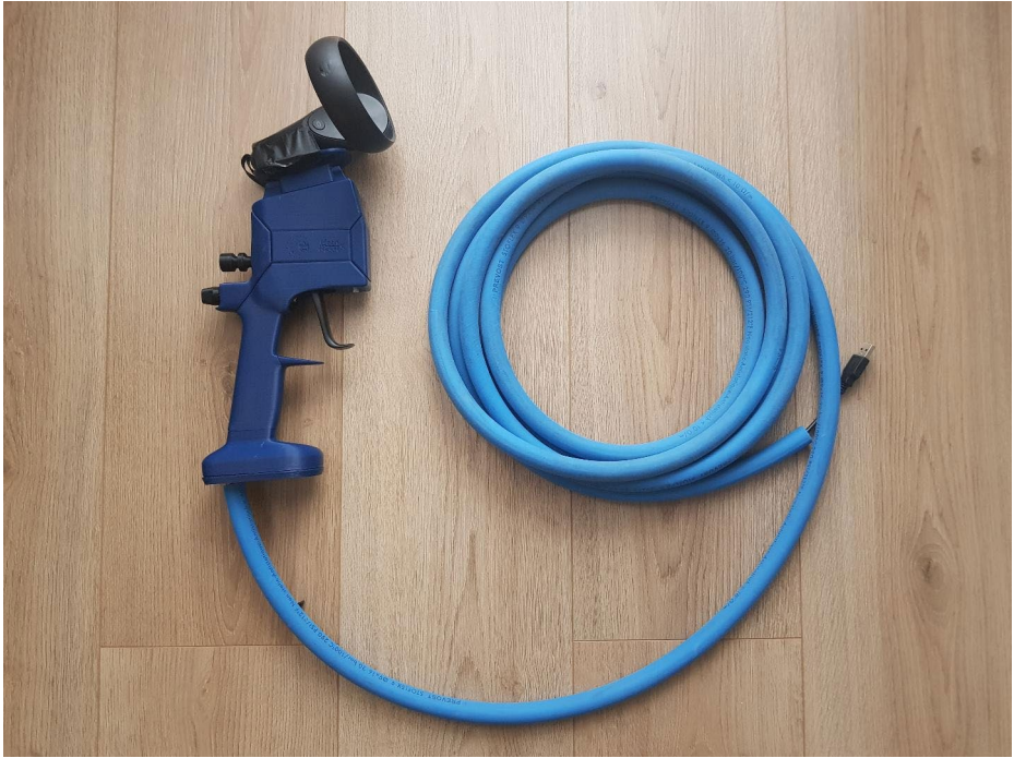
Fig. 4 The 3D printed spray gun
